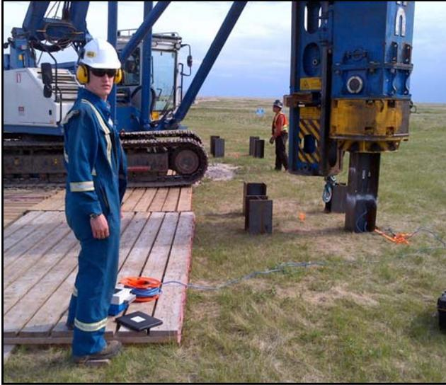
Dynamic load testing using **Pile Driving Analyser (PDA)** equipment is a high-strain non-destructive load test method which can be performed during or after pile installation using conventional pile driving equipment. This test can be applied to driven steel, driven timber and even concrete piles (eg. pre-stressed driven concrete piles, drilled shafts, auger cast piles).
