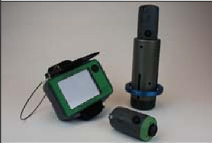
**Pile Integrity Testing (PIT)** is a low-strain and non-destructive integrity test method which only involves the impact from a small hand-held hammer. This low-strain test can be applied to any concrete piles (eg. Pre-stressed concrete piles, drilled shafts, auger cast piles, concrete filled pipe piles). Acceleration and stress wave which generated by the impact of small hand held hammer is the input of this test method.
